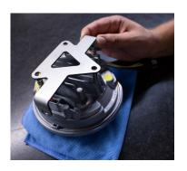
8. Take your J.W. Speaker lamp and place it face down on the lens on a protected surface so the lens does not get scrateched. Put the rubber ring around the housing of the light.
