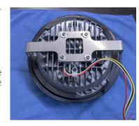
9. Place the lamp/ bracket assembly in the trim ring. Place the M5 bolt through the trim ring, and into the JWS bracket. Tighten the M5 bolt with the appopriate hex wrench.
