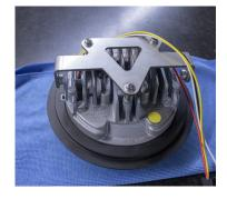
9. Place the lamp/ bracket assembly in the trim ring. Take the M5 bolt, bushing, and the lock washer, and assemble them as seen in photo. Tighten the M5 bolt with the appopriate hex wrench.
