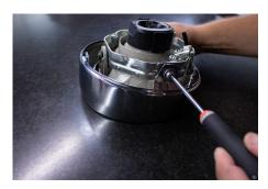
5. Remove the lamp assembly from the trim ring. the lamp assembly can only be removed by sliding it out of the ring, lens forward.
