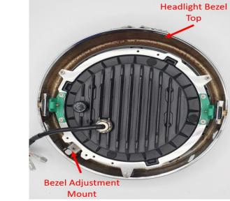
**Step 5:** Slide the Headlight assembly in the Suzuki bezel from the back side. Line up the side mount holes with the bezel mounts. Use the existing hardware from the stock headlight. Have the T-Nuts facing each other. You can use Blue Thread lock on the stock hardware.
