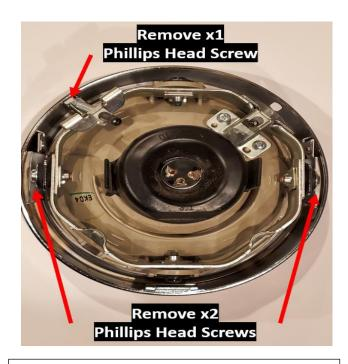
**Step 4:** Remove the adjustment bracket by removing two Philips head screws. Remove one of the adjustment screws from the bezel. Keep the screws and T-Nuts for later use. Keep the grommets in the bezel mounts.
