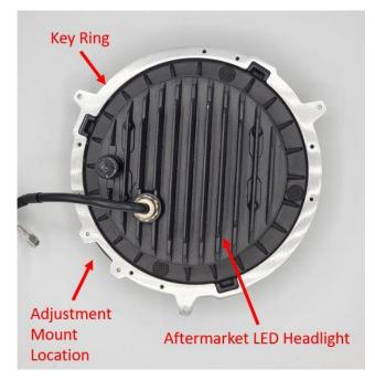
**Step 1:** Take the Key Ring and align the three keyways and keys of the LED Headlight. The LED headlight should be facing up and the adjustment mount location to be positioned to the bottom left.
