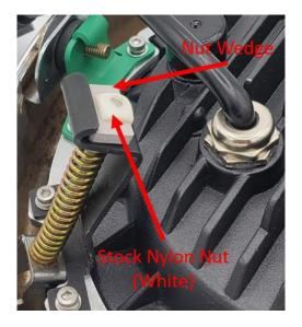
**Step 8**: Now take the stock M4 long adjustment screw and guide it through the bezel hole and the bezel adjustment hole. Then pass it through the spring. Do not pass it all the way through the adjustment mount yet.
