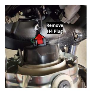
**Step 3:** Remove the Headlight assembly by slightly twisting and pulling on the bezel. Then unplug the H4 plug.
