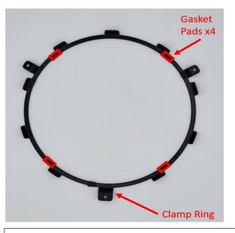
**Step 2:** Apply the 4 provided EPDM gasket cutouts to the bottom side (tabs facing up) of the clamp ring in the approximate locations described above. This will cushion the LED headlight in the setup and reduce vibration. When applying use pressure for 20 seconds. This is an optional step.
